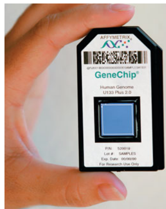
FIGURE 22-18 A commercially available DNA microarray, called a GeneChip, marketed by Affymetrix, Inc. This microarray can be used to analyze expression for approximately 50,000 RNA transcripts. It contains 22 different probes for each transcript and allows scientists to simultaneously assess the expression levels of most of the genes in the human genome.
