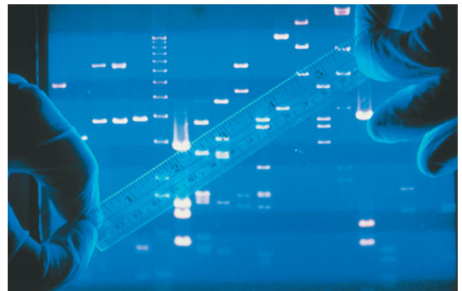
FIGURE 20–10 An agarose gel containing separated DNA fragments stained with the DNA-binding dye (ethidium bromide) and visualized under ultraviolet light. Smaller fragments migrate faster and farther than do larger fragments, resulting in the distribution shown. Molecular techniques involving agarose gel electrophoresis are routinely used in a wide range of applications.
