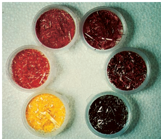
FIGURE 22.27 Mixed crystals of two semiconductors with different band gaps, CdS (yellow) and CdSe (black), show a range of colors, illustrating a decrease in the band gap energy as the composition of the mixture becomes richer in Se.
