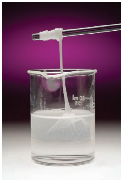
FIGURE 23.5 Hexamethylenediamine is dissolved in water (lower layer), and adipyl chloride, a derivative of adipic acid, is dissolved in hexane (upper layer). At the interface between the layers, nylon forms and is drawn out onto the stirring bar.
