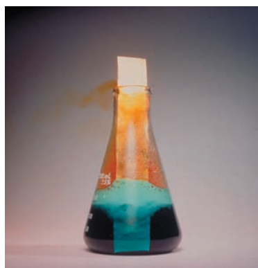
FIGURE 9.8 When copper metal is immersed in concentrated nitric acid, the copper is oxidized and an aqueous solution of blue copper(II) nitrate forms. In addition, some of the nitrate ion is reduced to brown gaseous nitrogen dioxide, which bubbles off.
