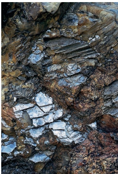
FIGURE 22.4 Naturally occurring muscovite mica. The mechanical properties of crystals of mica are quite anisotropic. Thin sheets can be peeled off a crystal of mica by hand, but the sheets resist stresses in other directions more strongly. Transparent, thin sheets of mica, sometimes called isinglass, have been used for heat-resistant windows in stoves or in place of window glass.
