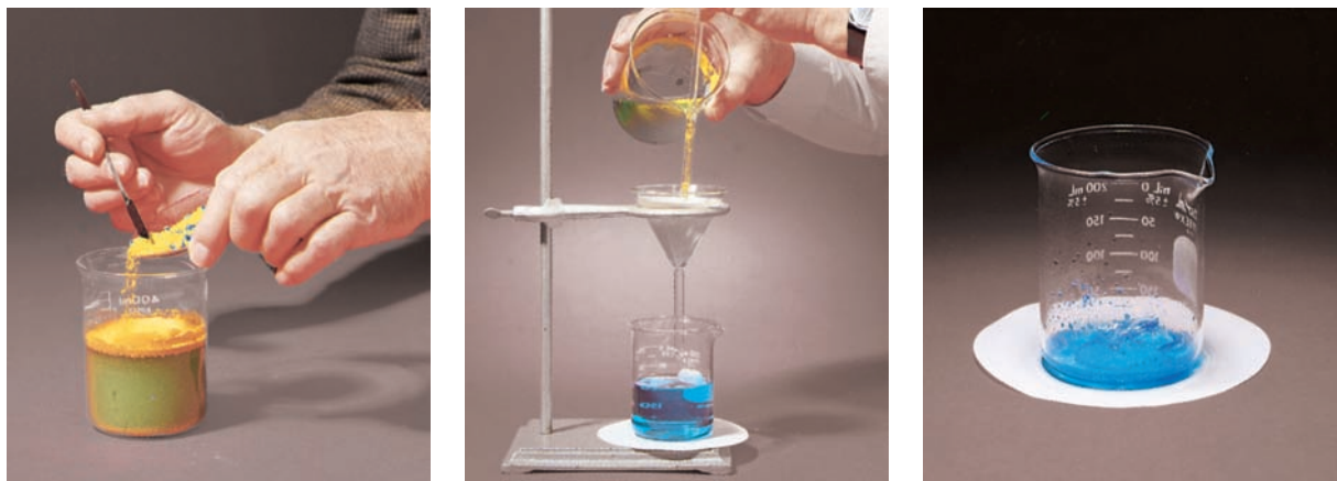
FIGURE 1.4 (a) A solid mixture of blue \text{Cu}(\text{NO}_3)_2 \cdot 6\text{H}_2\text{O} and yellow \text{CdS} is added to water. (b) Although the \text{Cu}(\text{NO}_3)_2 \cdot 6\text{H}_2\text{O} dissolves readily and passes through the filter, the \text{CdS} remains largely undissolved and is held on the filter. (c) Evaporation of the solution leaves nearly pure crystals of \text{Cu}(\text{NO}_3)_2 \cdot 6\text{H}_2\text{O} .
