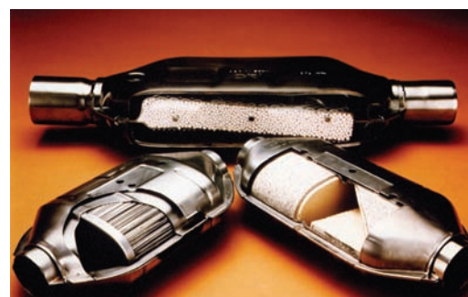
FIGURE 18.16 (a) The arrangement of a catalytic converter used to reduce automobile pollution. (b) Cutaway views of several catalytic converters showing different structures for organizing metal catalysts, platinum, palladium, and rhodium on different substrates and supports. A steel-alloy heating element raises the temperature to 400^\circ C in seconds, activating the catalysts and reducing the pollution emitted in the first minutes after the car is started.
