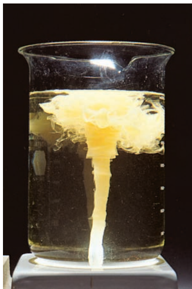
FIGURE 16.15 The “orange tornado” is a striking demonstration of the effects of complex ions on solubility. A solution is prepared with an excess of I^{-}(aq) over Hg^{2+}(aq) so that the Hg^{2+} is complexed as HgI_3^{-} and HgI_4^{2-} . A magnetic stirrer is used to create a vortex in the solution. Addition of a solution containing Hg^{2+} down the center of the vortex then causes the orange solid HgI_2 to form in a layer at the edges of the vortex, giving the tornado effect.
