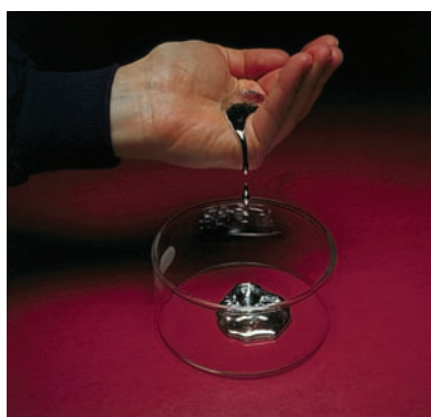
FIGURE 21.21 Solid gallium has a low melting point, low enough to melt from the heat of the body.
