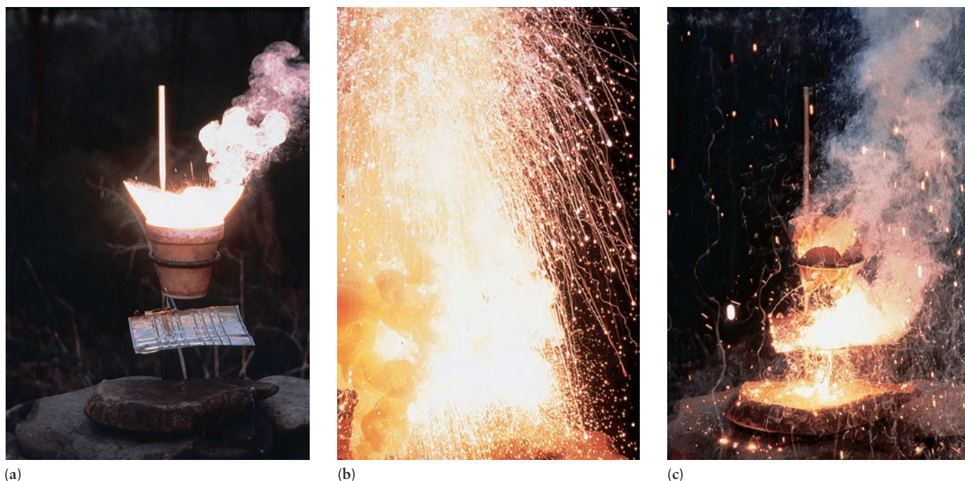
FIGURE 12.11 The thermite reaction, 2 \text{Al}(s) + \text{Fe}_2\text{O}_3(s) \longrightarrow 2 \text{Fe}(s) + \text{Al}_2\text{O}_3(s) , is among the most exothermic of all reactions, liberating 16 kJ of heat for every gram of aluminum that reacts. (a) A piece of burning magnesium acts as a source of ignition when inserted into a pot containing a finely divided mixture of aluminum powder and iron(III) oxide. (b) After the ignition, the reaction continues on its own. (c) Enough heat is generated to produce molten iron, which can be seen flowing out of the broken pot onto the protective mat and the bottom of the stand.
