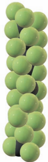
FIGURE 23.7 A model of the molecular structure of Teflon shows that the fluorine atoms shield the carbon chain very effectively. Note that the chain must twist to accommodate the bulk of the fluorine atoms, completing a full spiral every 26 C atoms along the chain.
