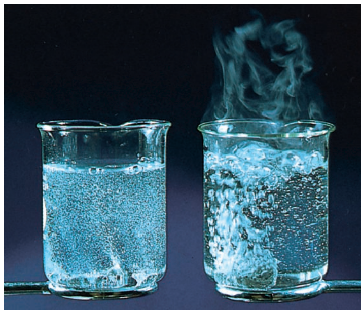
FIGURE 18.1 The rate of reaction of zinc with aqueous sulfuric acid depends on the concentration of the acid. The dilute solution reacts slowly (left), and the more concentrated solution reacts rapidly (right).
