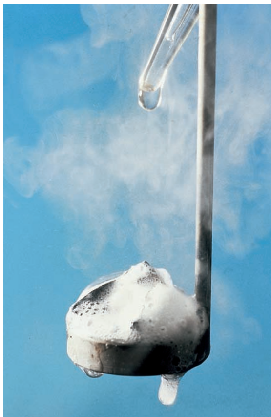
Gaseous nitrogen dioxide is generated by the reaction of copper with nitric acid.
