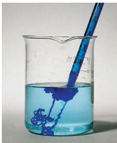
FIGURE 23.4 Filter paper (cellulose) will dissolve in a concentrated ammonia solution containing [\text{Cu}(\text{NH}_3)_4]^{2+} ions. When the solution is extruded into aqueous sulfuric acid, a dark blue thread of rayon (regenerated cellulose) precipitates.
