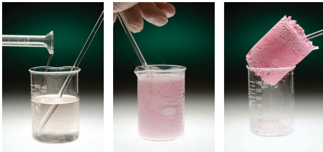
FIGURE 23.3 When a mixture of phenol ( \text{C}_6\text{H}_5\text{OH} ) and formaldehyde ( \text{CH}_2\text{O} ) dissolved in acetic acid is treated with concentrated hydrochloric acid, a phenol-formaldehyde polymer grows.
