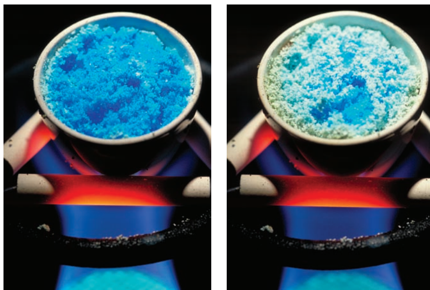
FIGURE 8.11 Hydrated copper(II) sulfate, \text{CuSO}_4 \cdot 5\text{H}_2\text{O} , is blue (left), but the anhydrous compound, \text{CuSO}_4 , is greenish white (right). A structural study of the solid compound demonstrates that four of the water molecules are closely associated with the copper and the fifth is not. Thus, a better representation of the hydrated compound is [\text{Cu}(\text{H}_2\text{O})_4]\text{SO}_4 \cdot \text{H}_2\text{O} .
