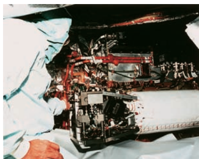
FIGURE 17.11 A hydrogen–oxygen fuel cell used on U.S. space missions.
