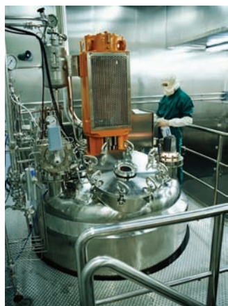
FIGURE 7.34 Fermentation tanks used in modern penicillin production.
